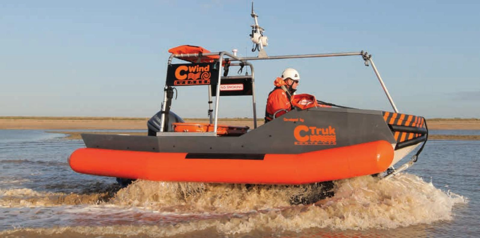
CTruk Avenger is an amphibious rescue and survey vehicle that can be carried on and launched from a CTruk 20T MPC or other mother ship.
