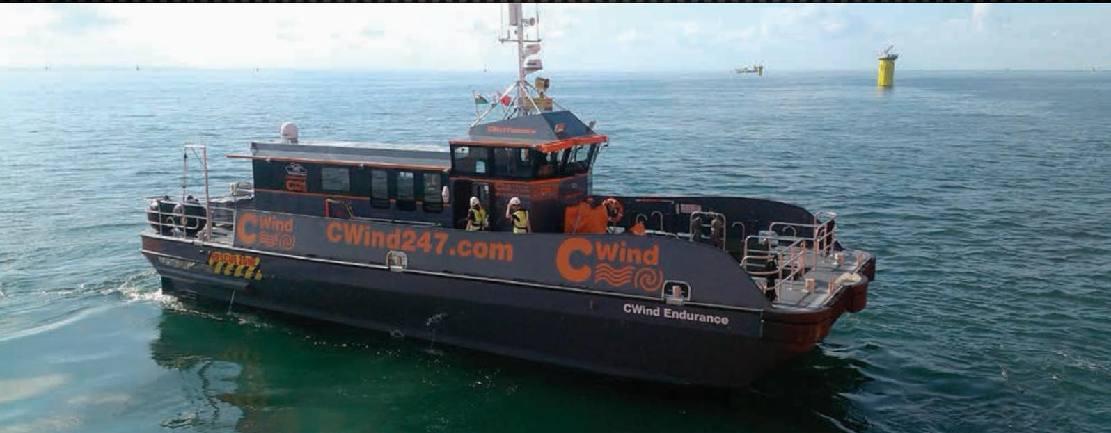
The SWATH20 (small waterplane area twin hull) design objectives were to dramatically improve the comfort of technicians transiting to offshore wind farms. Motions are approximately a quarter of those of conventional catamarans, significantly increasing the wave height limits for technician transfer.
